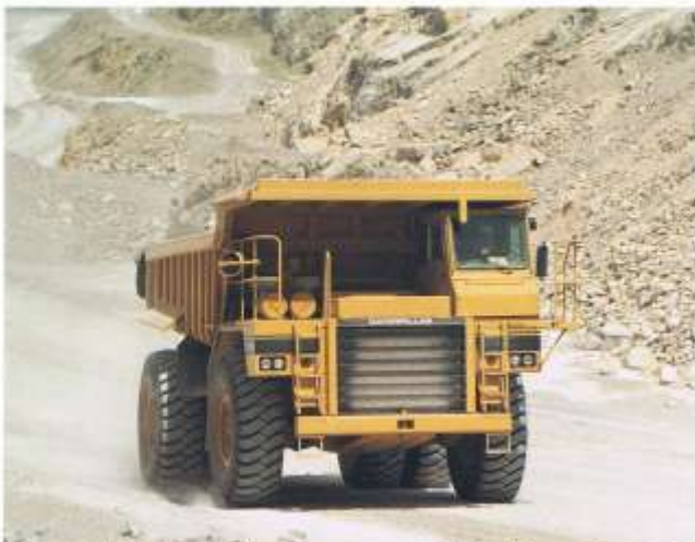
Steep grades put emphasis on horsepower and fuel efficiency. A good haul road maintenance program can cut equipment cost.
