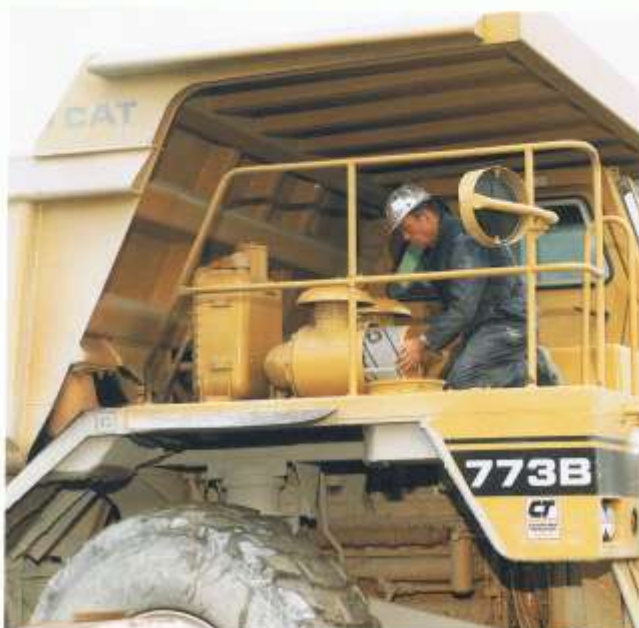
Easy access to routine maintenance points, from the ground or from platforms on the truck, helps keep maintenance hours and cost down.
