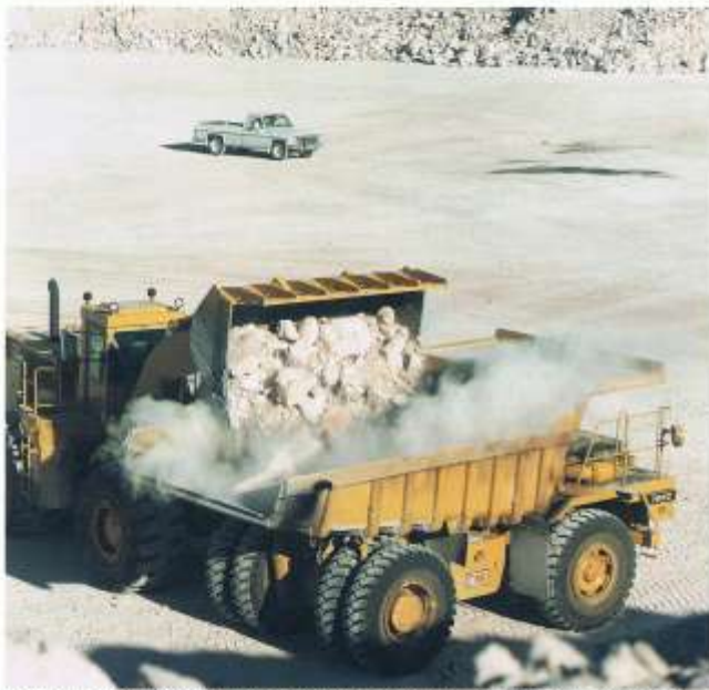
Modern trucks offer greater payload, performance, and fuel efficiency — plus improved cabs. A good match with the crusher and loader is the first requirement in truck selection.
